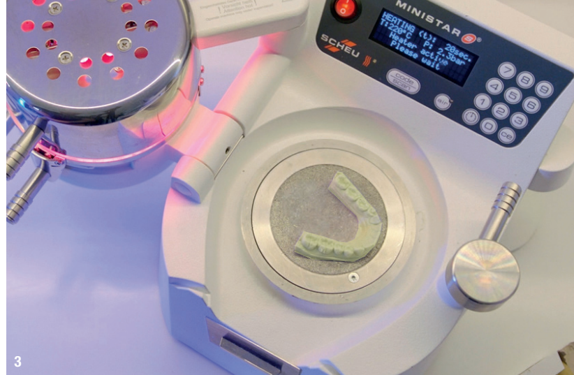
Fig.3: The MINISTAR S for vacuum forming.
